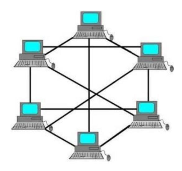
In a mesh topology, each computer system is connected directly to each of the others. Each node relays data for the network
