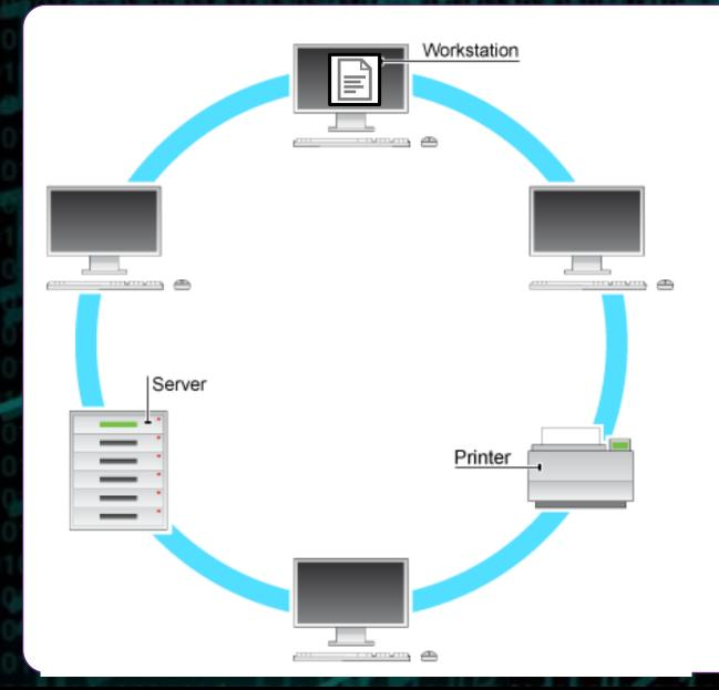
In a ring network, computer systems are connected in a ring or a loop.
