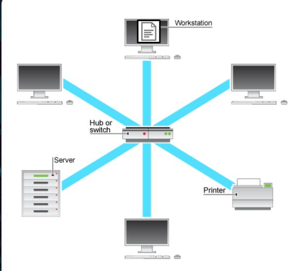
In a star network, each computer system is connected to a central node, also known as a hub or switch.
