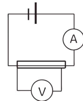
**Set up the apparatus as shown. Attach the first crocodile clip at 0cm. Attach the second crocodile clip at 10cm. Record the potential difference and the current. Connect the second crocodile clip at different lengths (20cm, 30cm) and repeat the process. Use the results to calculate resistance at different lengths, using the formula: resistance = potential difference ÷ current**
