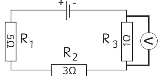
On the diagram, draw where a voltmeter could be positioned to measure the voltage through one of the components.
