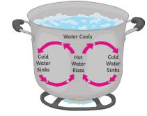
**Evaporation** occurs when heat energy from the surroundings (or a heat source) is transferred to water particles as kinetic energy. The particles begin to move more rapidly and can turn from a liquid into a gas.
