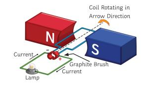
As the **current** flows (from negative to positive), the force produced in each side of the coil acts in **opposite directions**, causing the coil to **rotate** overall.
